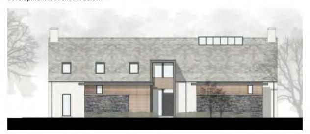
The apartments will be finished with a replica slate pitched roof, trocal flat roof (grey in colour); aluminium window frames and door frames (grey in colour); stone cladding where shown (brown/grey in colour); smooth render walls where shown (white/off-white in colour); select stone/brick walls where shown (grey in colour); board and batten cladding (larch or similar); precast concrete cills where shown; glass screens to balconies.
