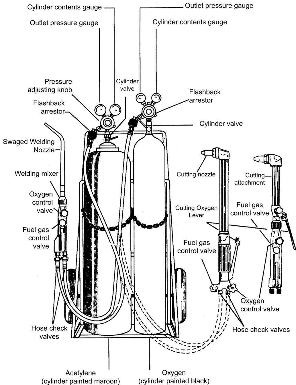
Typical equipment used in gas welding and allied processes
