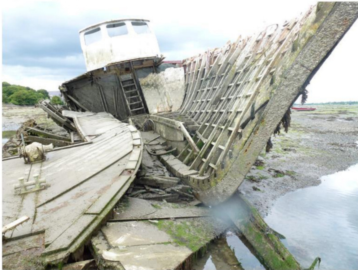
No.6 showing starboard side of hull missing. Keel still fitted
