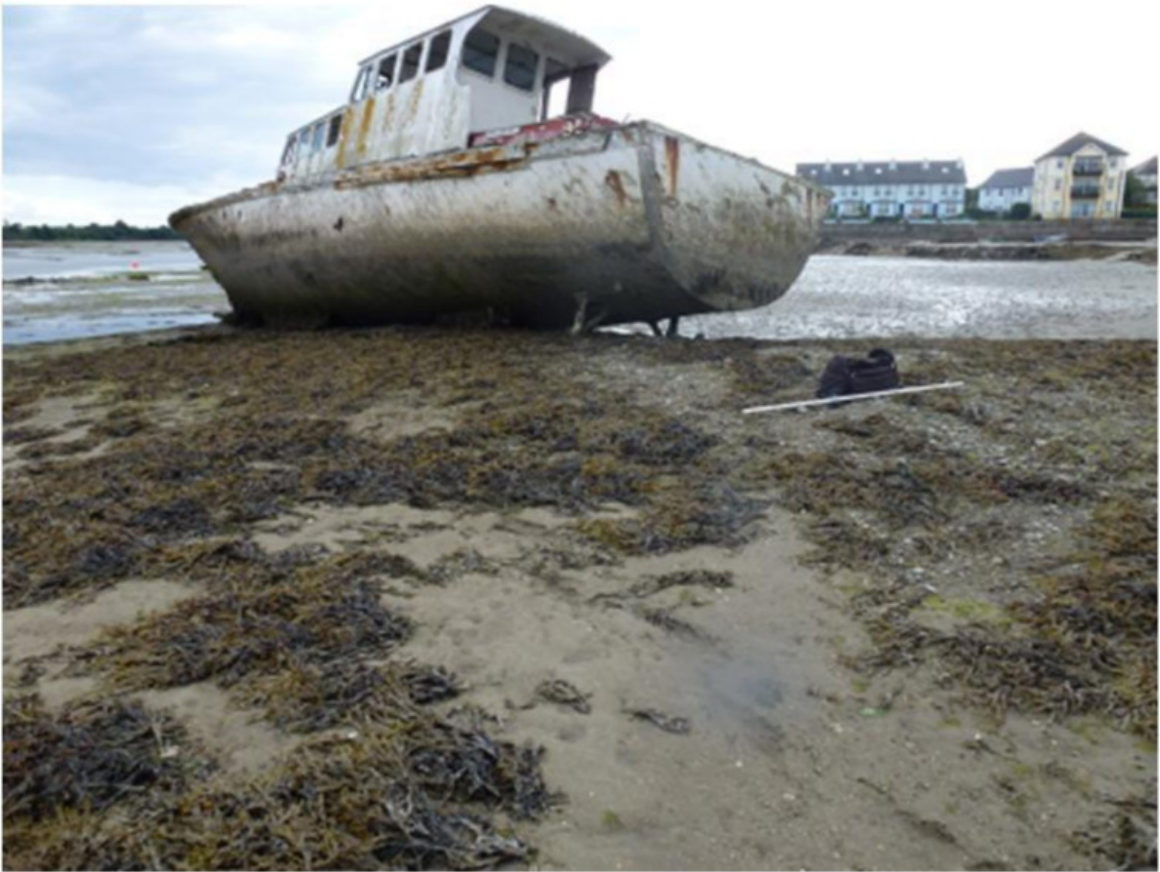
No.7 photo showing vessel sitting on shingles & sand. Aft section of the Keel is raised above the sand (convenient for sliding lifting sling under this part of the keel )
