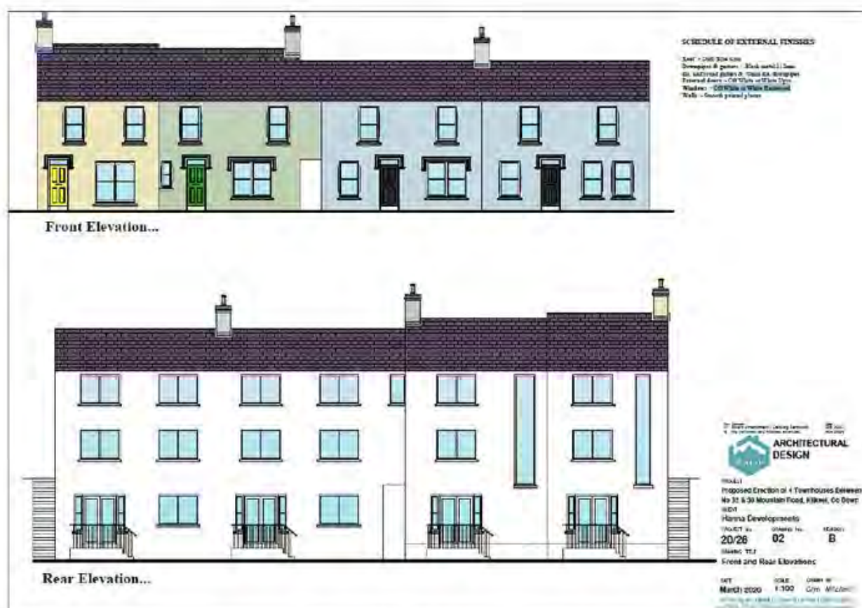
Proposed front and rear elevations
