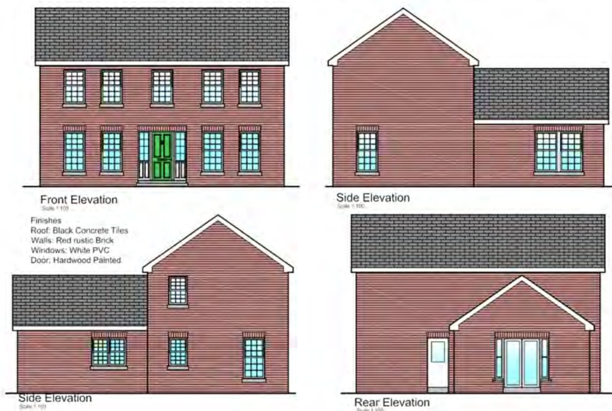
Figure 2: Proposed Elevations – Note No First Floor Windows in Southern or Eastern Elevation
