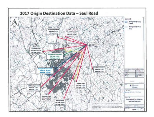
The origin destination data also provides a useful indication of traffic movements which could potentially re-route to use the Downpatrick Eastern Distributor Road which is highlighted in yellow.
