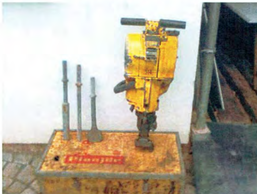
Pionjar deep overburden sampling device
